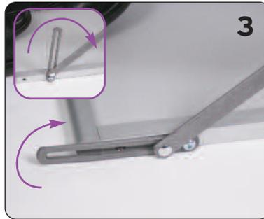
Whilst raising the unit note position of the pivot arms. To ensure correct assembly both pivot arms must rotate through 180 degrees.
